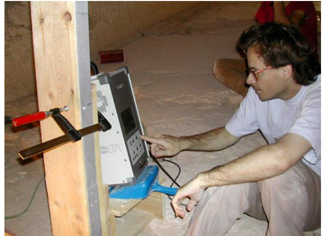
Figure 8. The Minolta 900 on a specially built rig allowing the scanner to remain perpendicular to the scanned surface (i.e., parallel with the surface normal of the resulting model).
