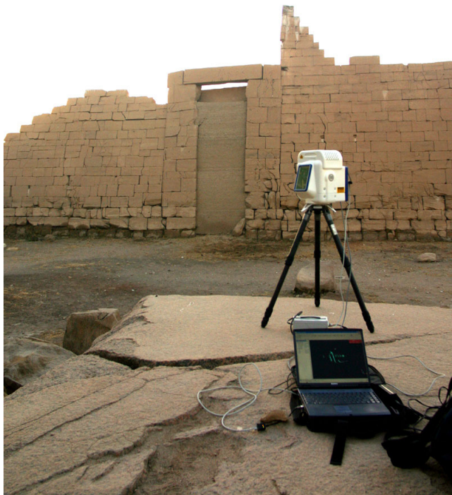
Figure 4. GS-100 and Control Computer.
