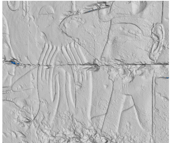
Figure 13. Example of data quality. The ideal surface characteristics of the KV7 walls allow clean, accurate optical triangulation data to be taken.
