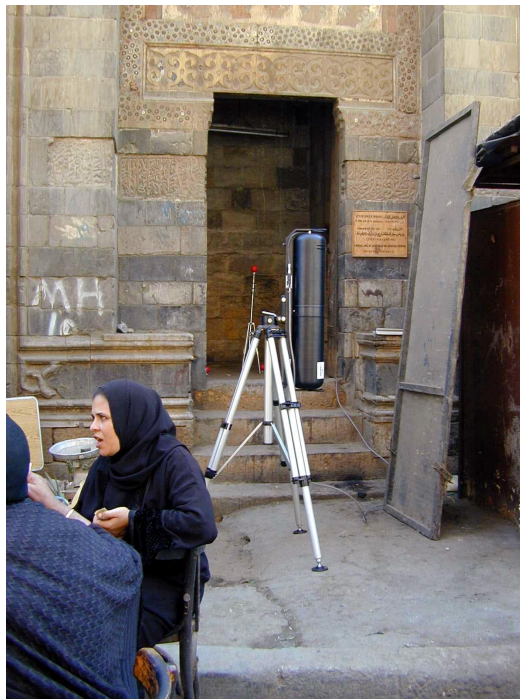
Fig. 2 – The laser scan sensor on site (positioned vertically); a red reference sphere is visible on its tripod.
