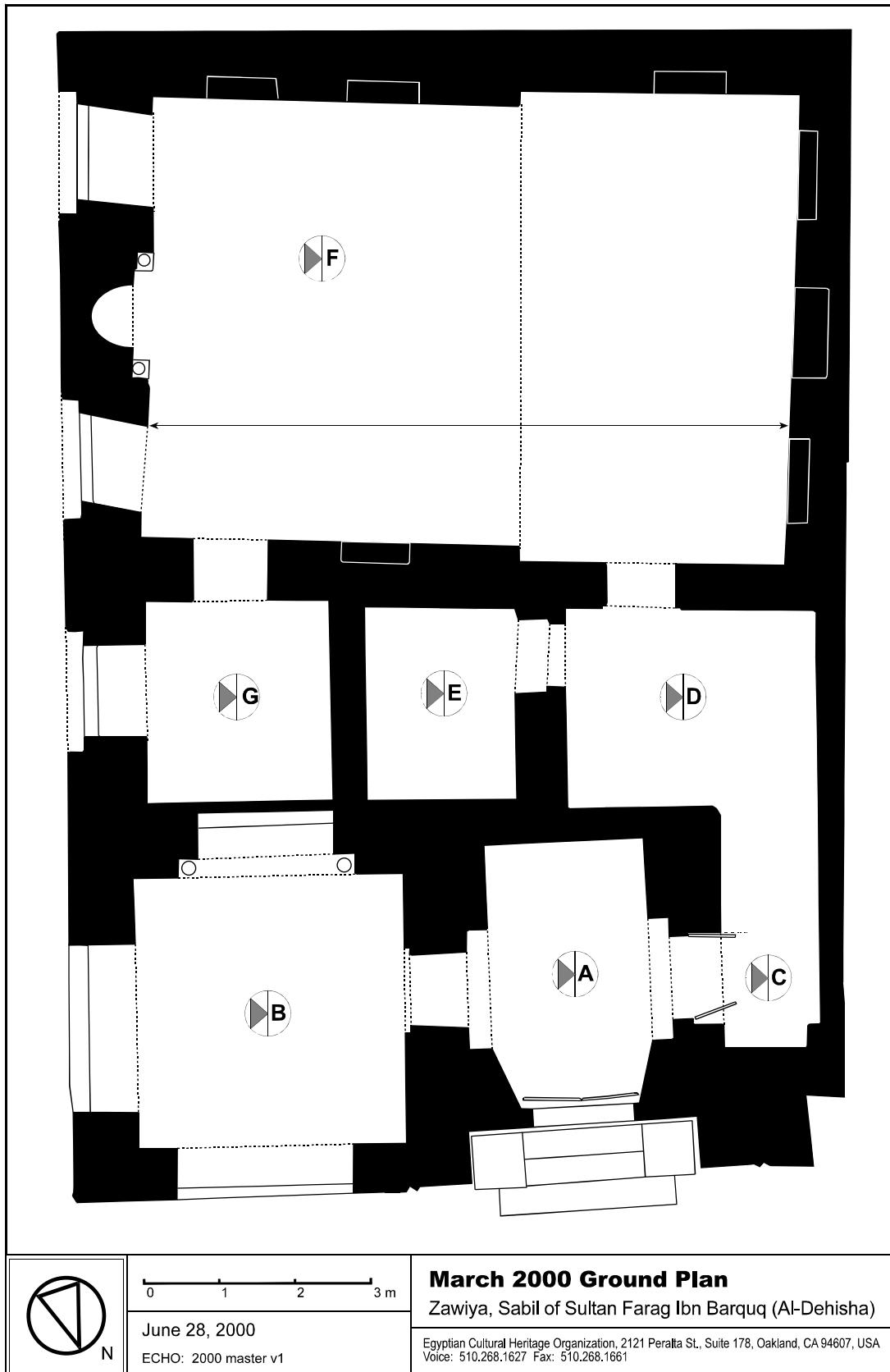
Fig. 7—Ground plan using March 2000 interior and exterior scan data
